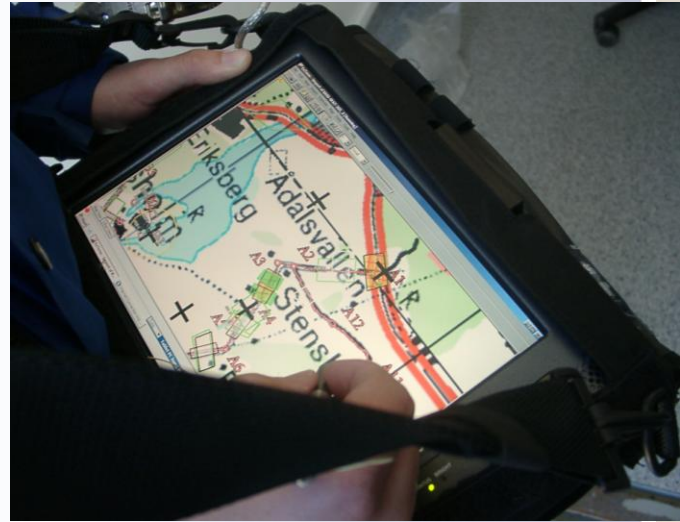
Two function buttons on the keypad have been programmed to zoom the display and to switch between the map view and task panel view.
